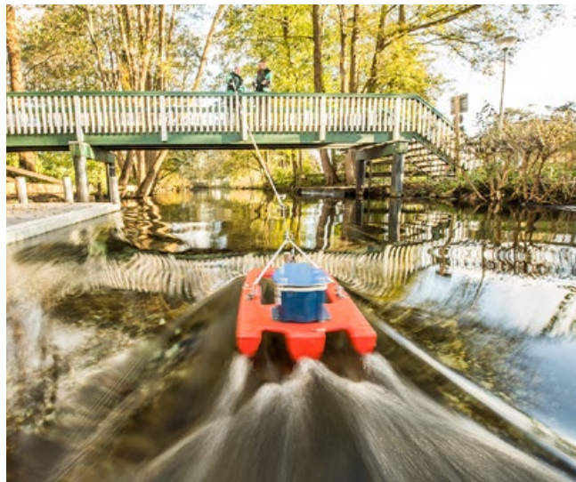
Measuring sensors are used to determine water levels in ground- and surface waters, and mobile ultrasonic measuring devices are employed to record the flow velocity in a body of water. Wave buoys continuously record the height of sea waves.
