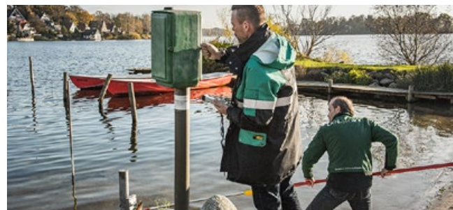
Measuring sensors are used to determine water levels in ground- and surface waters, and mobile ultrasonic measuring devices are employed to record the flow velocity in a body of water. Wave buoys continuously record the height of sea waves.
